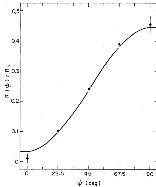
FIG. 2.  $R(\varphi)/R_0$  as a function of angle  $\varphi$  between polarization planes. Solid curve is the quantum-mechanical prediction calculated using measured average polarizer efficiencies, solid angles, and Hg isotopic abundances.
