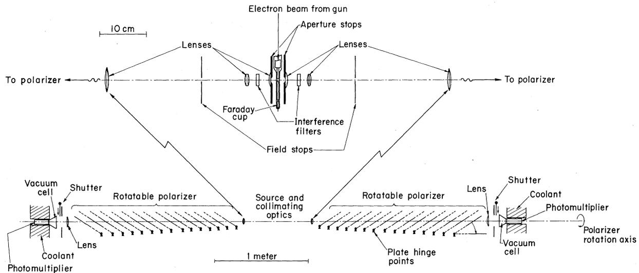
FIG. 1. Overall arrangement of apparatus, showing source and collimating optics (upper), and rotatable pile-of-plates polarizer assemblies and detectors (lower). Polarizer plates are removed for  $R_0$  measurement by folding them flat at their hinge points out of the optical path. The last plate on the right-hand side is shown in the removed position. Solid lines on plates depict glass plates; broken lines depict metal frames.
